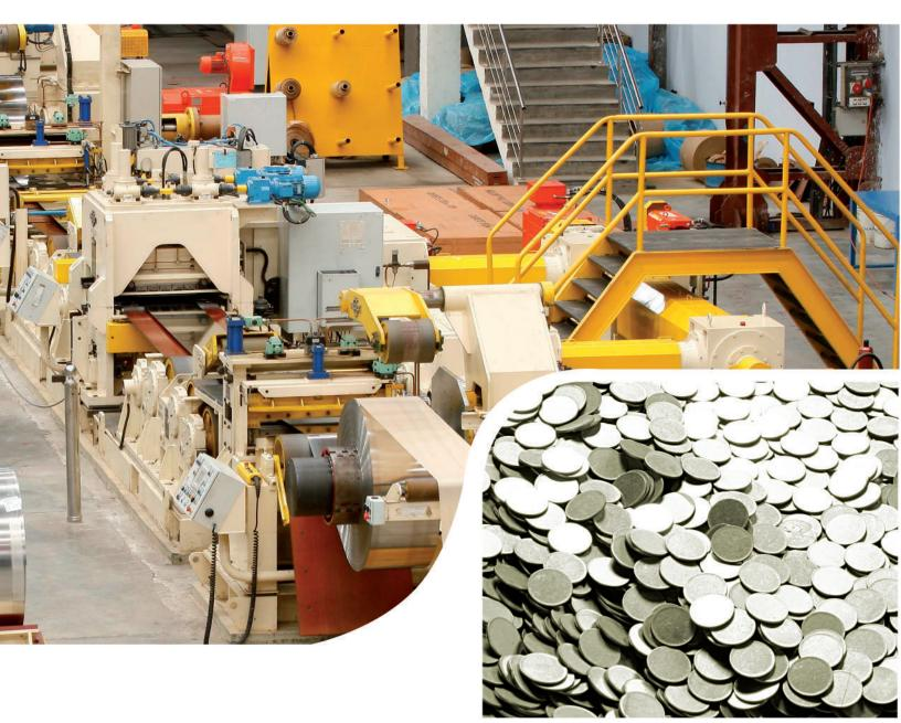
The razor blade cold rolled strips of up to 0.076mm thickness are produced in this complex and supplied to leading Indian and International razor blade manufacturers.
