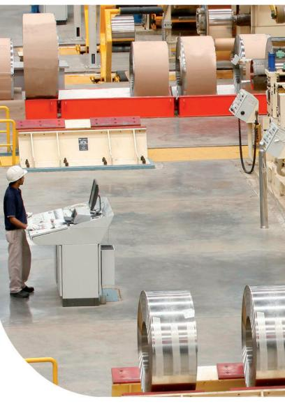
The Speciality Product Complex comprises of processing equipment, primarily for annealing, rolling and finishing. There is an option of using either a Bell Annealing or a Bright Annealing or even Pull-through Annealing, depending on the grade and finish, of Stainless Steel being produced.
